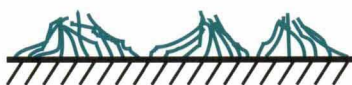
Figure 6.12 The mobility of deuterated silane monolayers on silical gel can be studied by solid state deuterium NMR spectroscopy. The degree of coating as well as the environment can be modified. The above models summarize the results. These modified silica surfaces are the most simple models for receptors of apolar molecules. The unique advantage of these probes is the large quantity of monolayer in a small volume.
